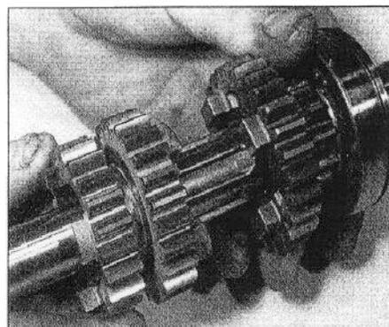
26.17 Install the combined 3rd/4th gear pinion ...
