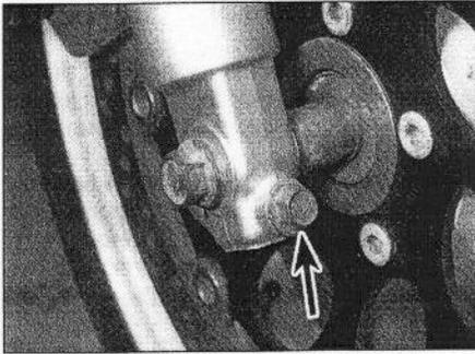
14.4a Slacken the axle clamp bolt (arrow) . . .
