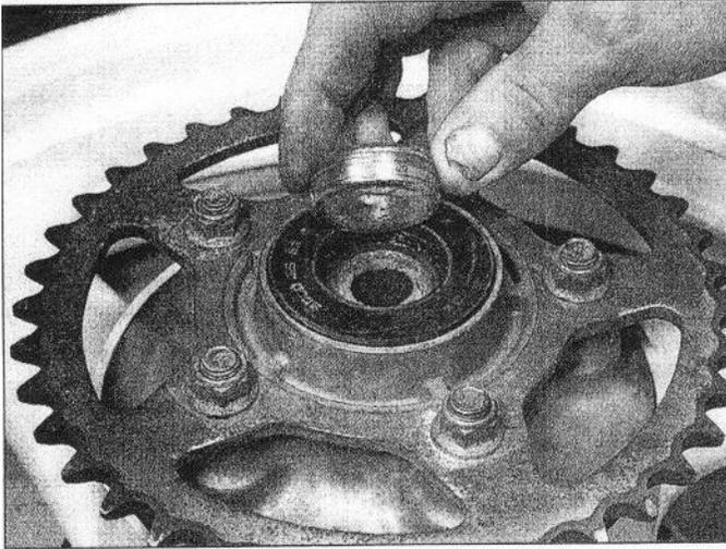
16.24a Remove the outer spacer . . .
