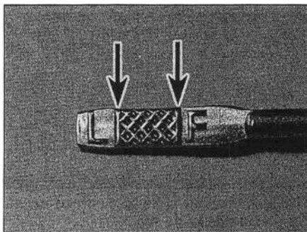
**3** Remove the dipstick and observe the level of the oil, which should be somewhere in between the upper 'F' and lower 'L' level lines (arrows).
