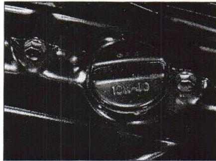
**1** Unscrew the oil filler cap from the right-hand side crankcase cover. The dipstick is integral with the oil filler cap, and is used to check the engine oil level.
