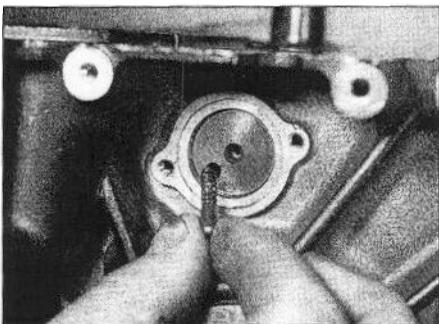
22.9a Install the spring and plunger ...
