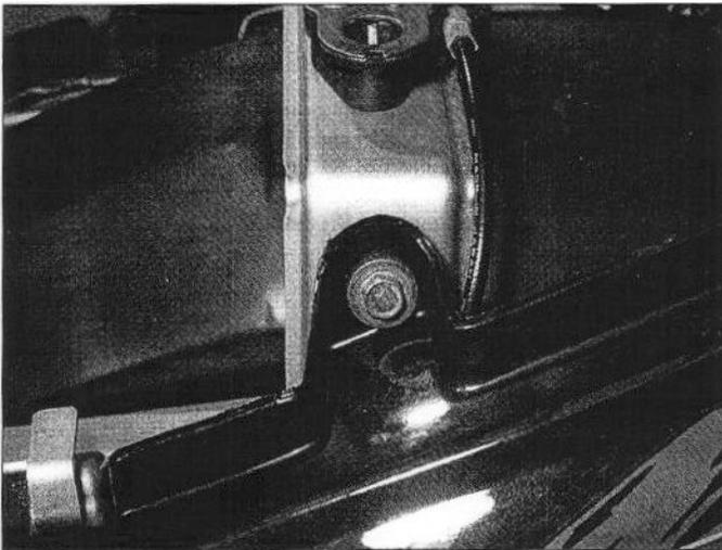
4.4a Each side panel is secured by a bolt . . .
