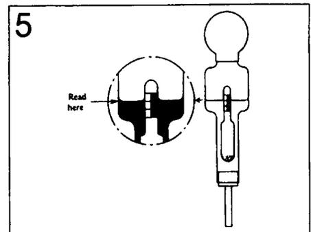
**Float-type hydrometer for measuring battery specific gravity**
