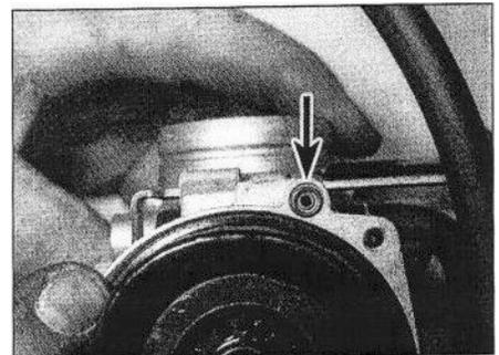
7.3 Remove the vacuum take-off pipe O-ring (arrow)
