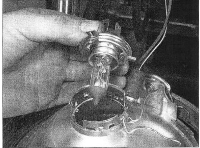
7.3b . . . and remove the bulb
