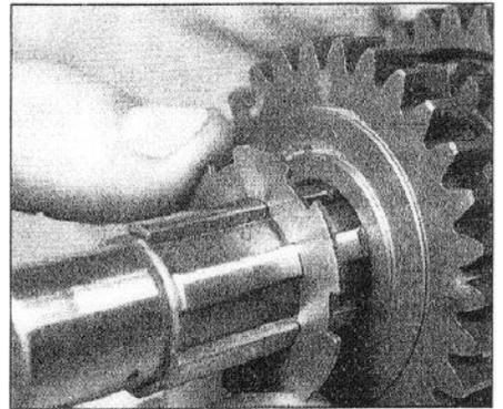
26.38c Install the inner lockwasher ...
