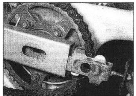
15.7 Install the chain adjusters into the swingarm
