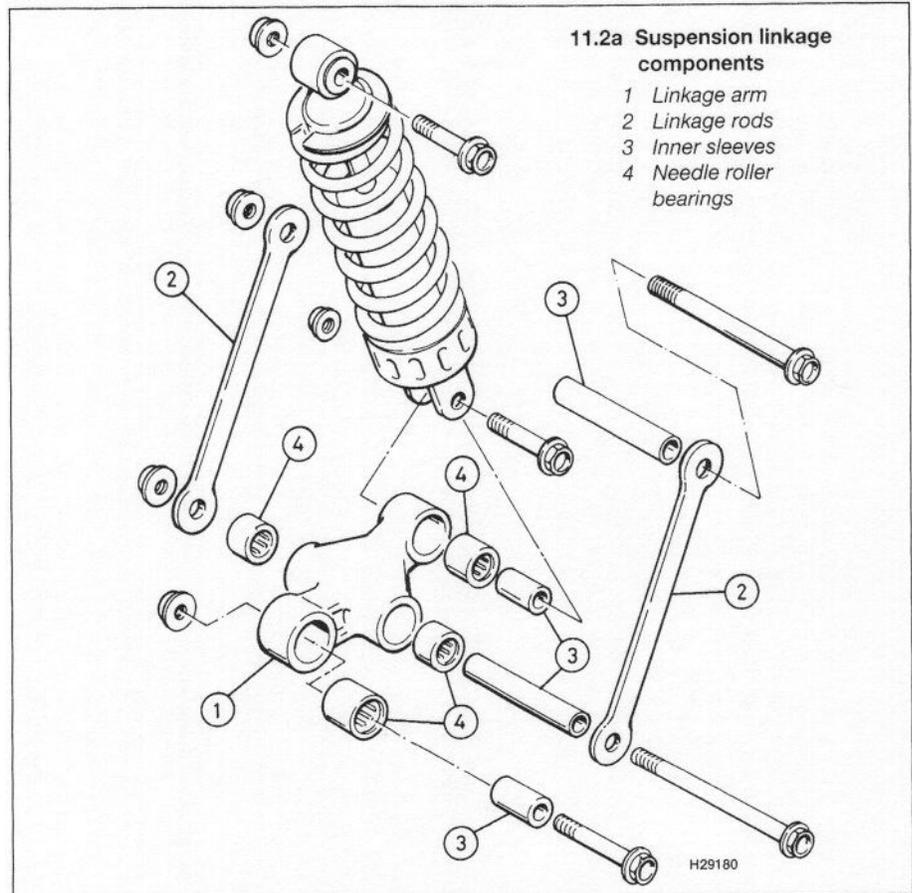
**11.2a Suspension linkage components**
