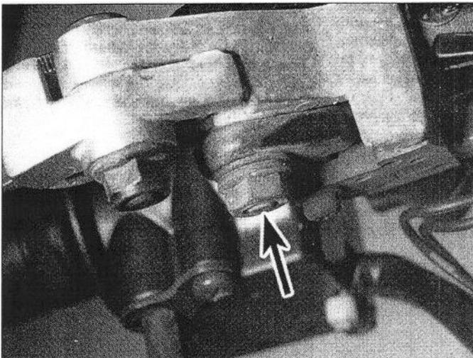
5.6a Remove the locknut (arrow) . . .
