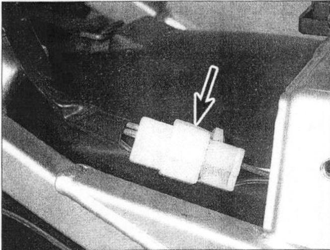
10.2 Disconnect the tail light wiring connector (arrow)
