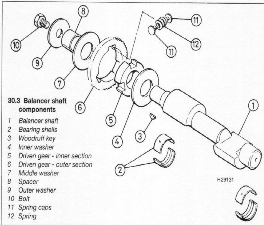
**30 Balancer shaft and bearings - removal, inspection and installation**
