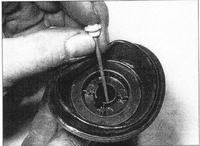
**7.5** Withdraw the jet needle assembly
