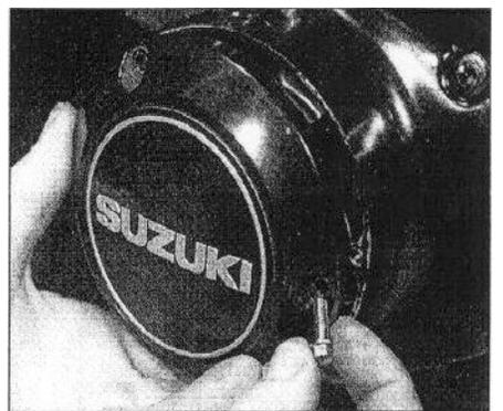
17.27 Install the pulse generator assembly cover
