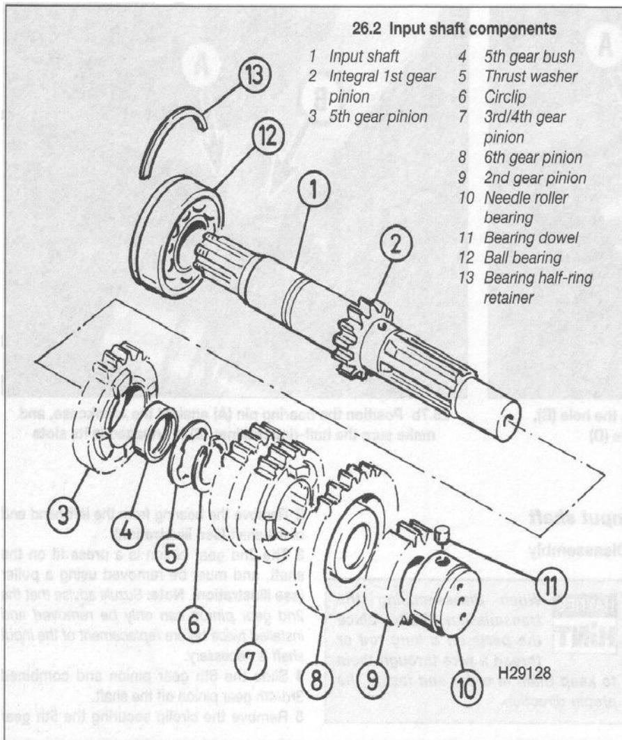
pinion, then slide the thrust washer and the pinion off the shaft, followed by the 5th gear bush.
