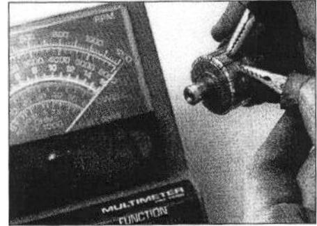
30.10a Continuity should exist between the commutator bars
