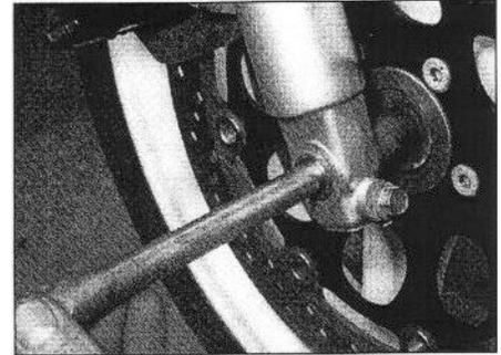
14.5 Withdraw the axle and remove the wheel
