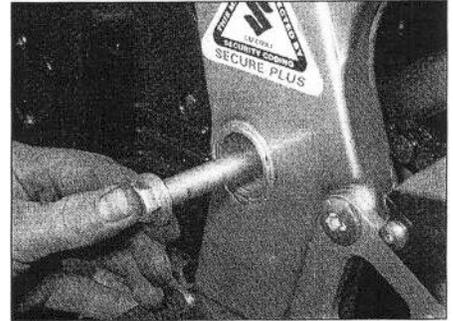
**13.6b ... and withdraw the swingarm pivot bolt**
