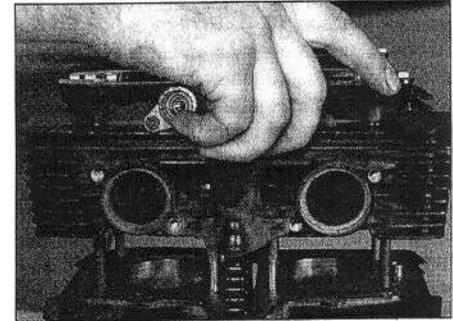
11.14 Lower the cylinder head onto the block
