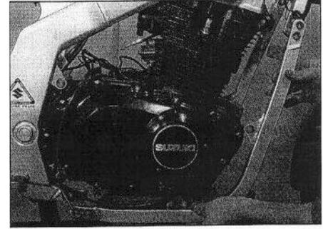
5.19b . . . and remove the frame downtube
