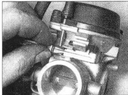
**9.1b** Secure the bar with the clips
