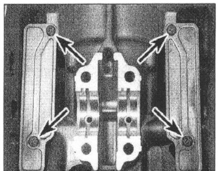
leaks will result. Check both crankcase halves very carefully for cracks and other damage.
