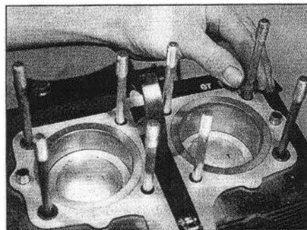
11.12 Fit a new O-ring around each stud
