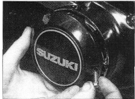
4.16 Install the pulse generator assembly cover
