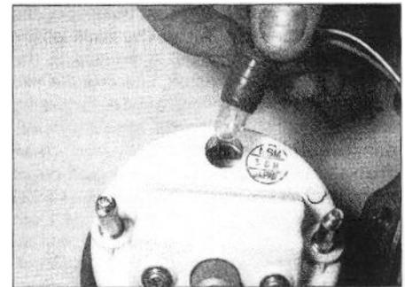
16.4b ... and remove the bulbholder
