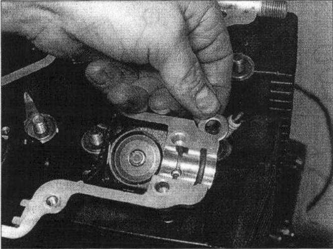
11.15a Fit new washers onto the studs . . .
