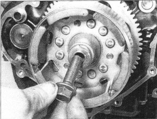
33.8b Install the rotor bolt . . .
