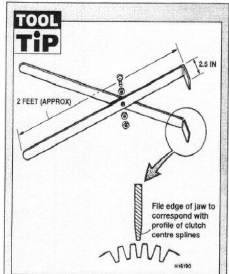
A clutch centre holding tool can easily be made using two strips of steel bent over at the ends and bolted together in the middle
