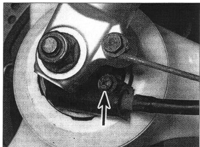
14.2 Unscrew the speedometer cable retaining screw (arrow)
