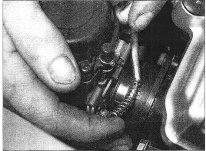
11.7 Fit the nipple into the linkage bar
