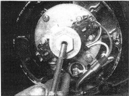
4.15b Install the rotor bolt . . .
