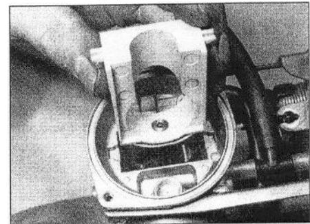
**7.9** Withdraw the piston guide and needle jet
