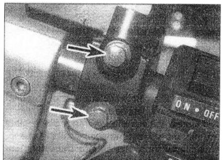
5.2 Front brake master cylinder clamp bolts (arrows)
