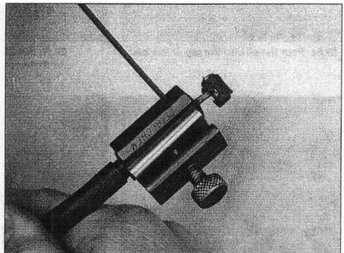
28.3 Lubricating a cable with a pressure lubricator
