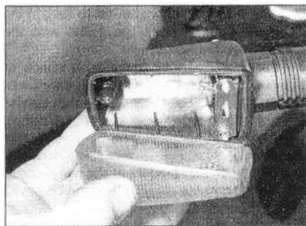
11.1b ... and remove the turn signal lens
